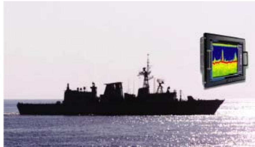
Marport's Software Defined Sonar transceivers will be used to upgrade the depth sounders on the Canadian Navy's Halifax class frigates. The technology insertion program will replace obsolete electronics while maintaining an interface to the original wet-end transducers.
