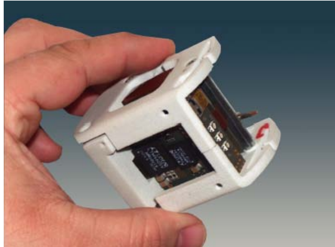
The SeaFire® acoustic modem is a robust underwater communication system designed to meet demanding requirements for undersea ISR. In addition to underwater telemetry, the compact electronics module incorporates a SDHC card data logger as well as onboard sensing capabilities such as 3-axis inclinometer, temperature, depth, humidity including direct interfaces to external sensors.
